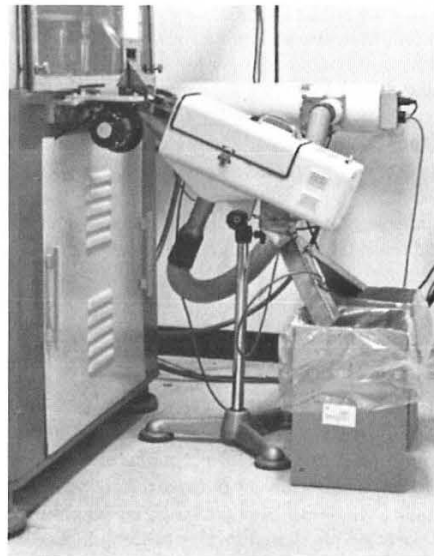
Fig. 7.47 Model 25 Manesty Tablet Deduster. Tablets leaving tableting machine are dedusted and passed into collection containers. (Courtesy of Eli Lilly and Company.)
