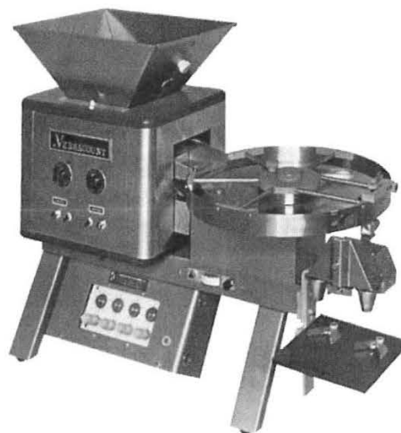
Fig. 7.18 Versacount Model automatic tablet and capsule counting and filling apparatus. (Courtesy of Production Equipment Co.)
