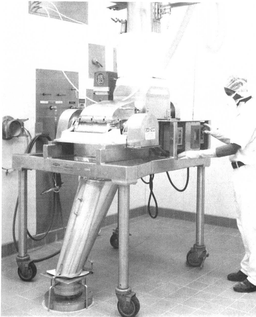
Fig. 7.42 Frewitt Oscillator or Fitz Mill utilized in the pulverization or granulation process. (Courtesy of Eli Lilly and Company.)
