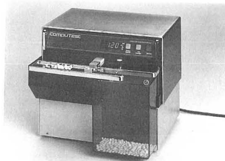
Fig. 7.32 CompuTest hardness tester, tests in Newtons, Kilopond, and Strong Cobb. Automatic or manually operated. tests up to 100 tablets per run. Integrated software stores product test programs. (Courtesy of Vector Corporation).
