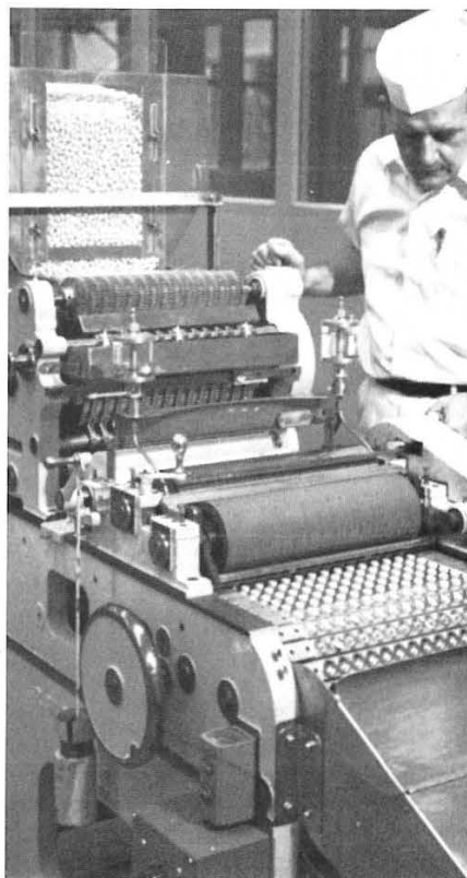
Fig. 7.52 Branding of coated compression tablets on a Hartnett branding machine. (Courtesy of The Upjohn Company.)
