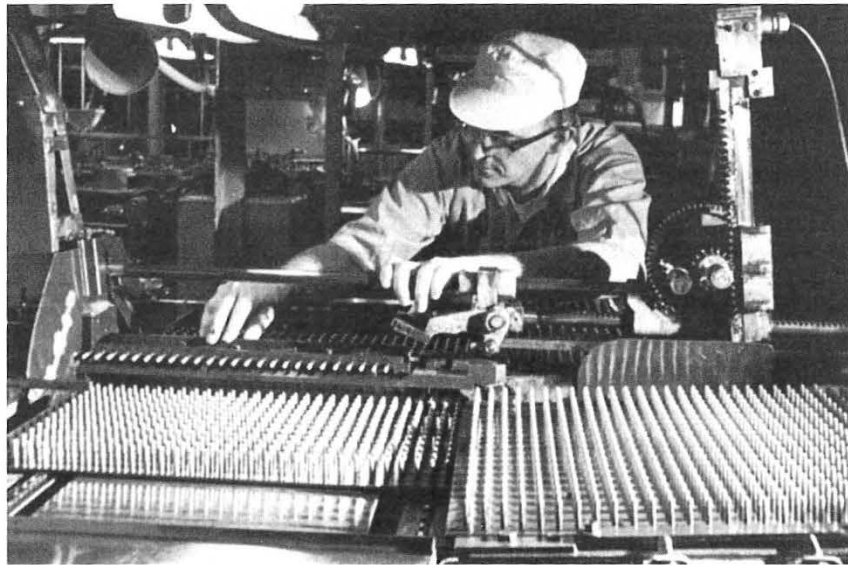
Fig. 7.2 Body of capsules and their caps are shown as they move through automated capsule-making machine. Each machine is capable of producing 30,000 capsules per hour. It takes a 40-minute cycle to produce a capsule. (Courtesy of SmithKline Beecham.)
