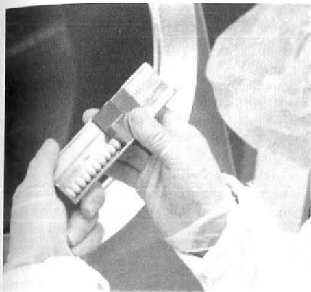
Fig. 7.51 Tablet gauge used to measure the size of coated tablets. (Courtesy of Eli Lilly and Company.)
