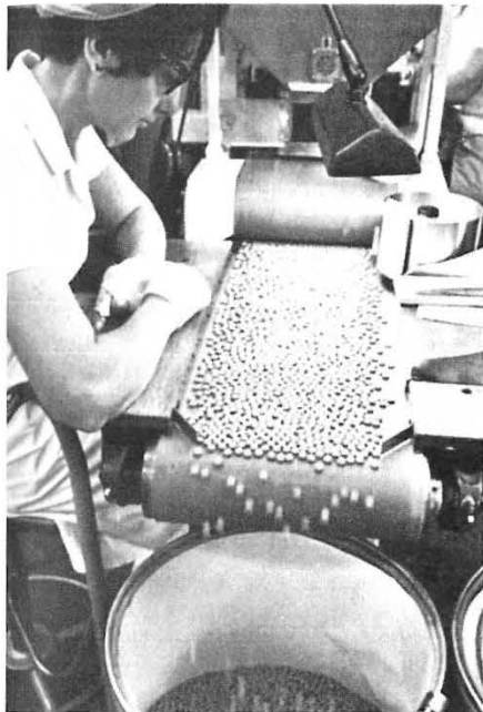
Fig. 7.56 Checking for physical imperfections in coated tablets. (Courtesy of Smith, Kline & French.)
