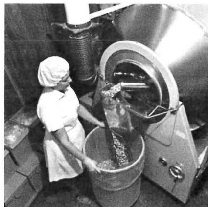
Fig. 7.14 Cleaning and polishing hard filled capsules using the Accela-Cota apparatus. (Courtesy of Eli Lilly and Company.)
