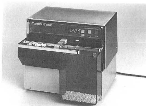
Fig. 7.32 CompuTest hardness tester; tests in Newtons, Kilopond, and Strong Cobb. Automatic or manually operated. tests up to 100 tablets per run. Integrated software stores product test programs. (Courtesy of Vector Corporation).
