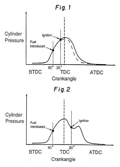
Figures 1 and 2 depict graphs showing the cylinder pressure-crankangle characteristics for a typical direct injected two-stroke internal combustion
