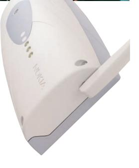
feature. AutoPIN means inserting the PIN code only once after a power cut, Nokia 20 relays the PIN code automatically. Normal GSM encryption and security codes are also supported in Nokia 20.
