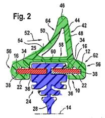
Figure 2 of the '136 patent depicts a cross-sectional view of a windshield wiper blade embodiment, with elastic rubber wiper strip 24 highlighted in blue, resilient support element 12 in red, and wind deflection strip 42 in green. As shown in Figure 2 of the '136 patent, wind deflection strip 42 has two sides (48, 50) that diverge from common point 46, such that, in conjunction with wall 58, wind deflection strip 42 is generally triangular in cross section and has a hollow interior.
