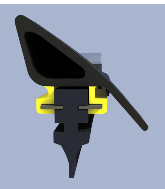
A wiper blade according to claim 1, naracterized in that wind deflection rip (42) is designed as a binary emponent whose longitudinal area ovided with the claw-like extensions 6) is made of a harder material than a ngitudinal area lying closer to the point (46).
