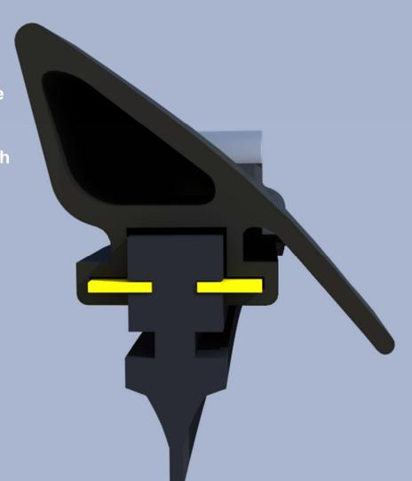
A wiper blade according to aim 1, characterized in that the apport element (12) includes to flexible rails (36) each of hich sits in a longitudinal notch 4) associated with it, spectively,...
