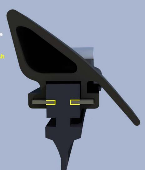
said longitudinal notches sing open toward the oposite lateral sides of the iper strip (24),...
