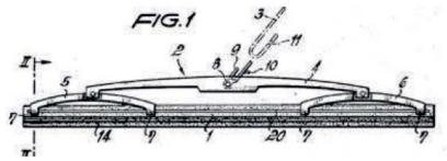
Figure 1 depicts a yoke-style wiper structure, having a large main rail 4 connected to two smaller rails 5, which in turn are connected to the wiper blade.
