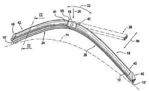
Figure 1 of the '905 patent depicts a beam-style wiper structure, in which the beam is attached along the entire length of the wiper.
