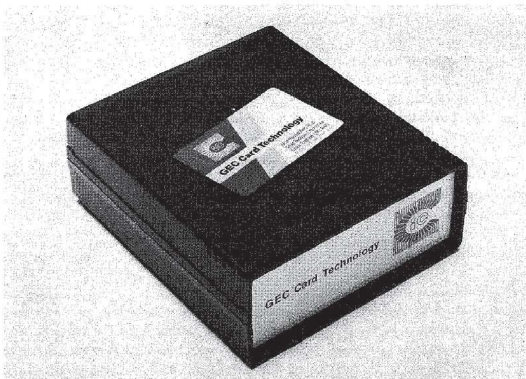
Fig. 3.3 The GEC ic Card and Coupler electronics are totally sealed making them ideal for use in harsh environments.
