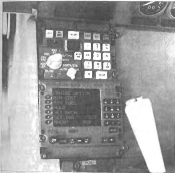
Figure 2. Typical installation of a 4-D Control and display Unit (CDU) in an L-1011.
