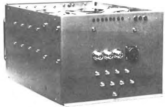
Fig. 3 TCAS Antenna Electronics Package
