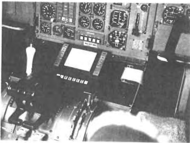
Fig. 2: The experimental pilot/link interface installed in the A 300B Airbus flight simulator.
