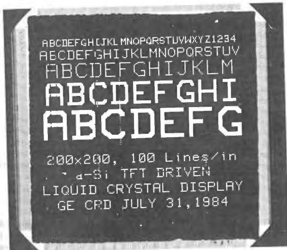
Figure 8 Photo of a 2 x 2 inch, 100 lines per inch \alpha -Si TFT Driven Transmissive LC Display
