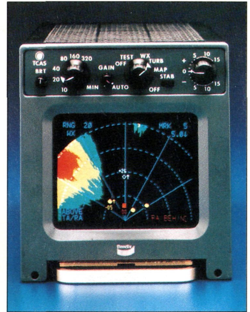
Weather radar can be combined with TCAS in a single display
