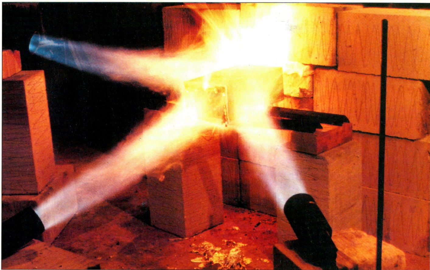
Flight recorders are tested to withstand extreme conditions to ensure information survival
