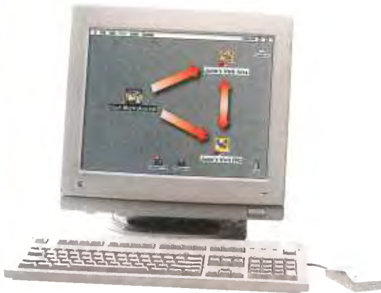
Using FullPress is completely intuitive. Users drag or scan original images into a FullPress shared volume, such as "Jamie's Work Area" or "Jamie's Work FPO" above. FullPress immediately creates "For Placement Only" (low-resolution) corollaries for use in page layout. Other users can also access the images (either the high-resolution original or the "For Placement Only" version) from their own Macs.
