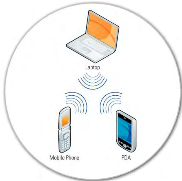
Figure 2-2. Bluetooth Ad Hoc Topology
