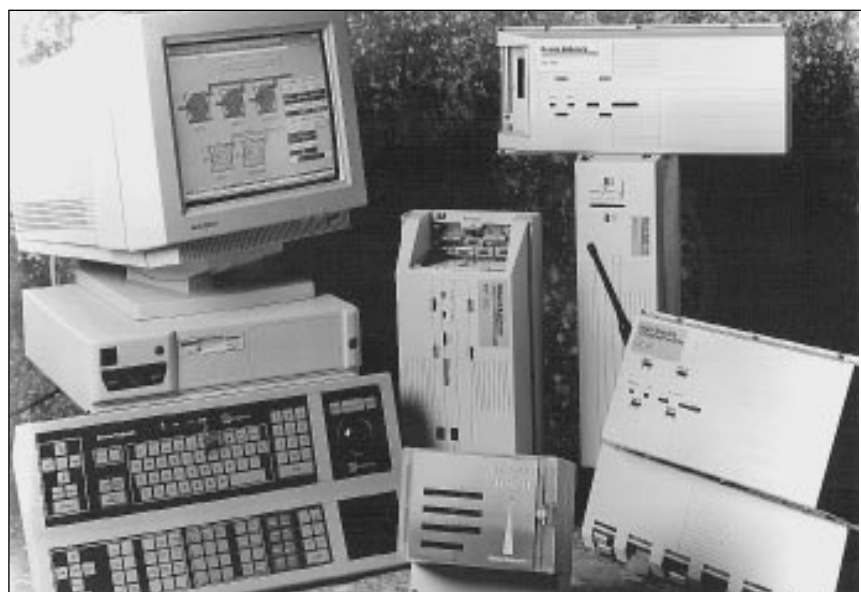
Bristol Babcock's Spacenet 3000 control and command station with Enterprise workstation and products from Bristol Babcock's Network 3000 process control range
