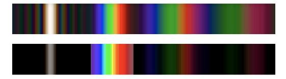
The solution is to employ the fact that gratings are most efficient when the rays emerge from the grating as if by direct reflection. By creating tilted facets, or a *blaze*, in the grating, as shown in figure 97, it is possible to direct the majority of the light ( $\sim 70\%$ ) into the order of interest.
