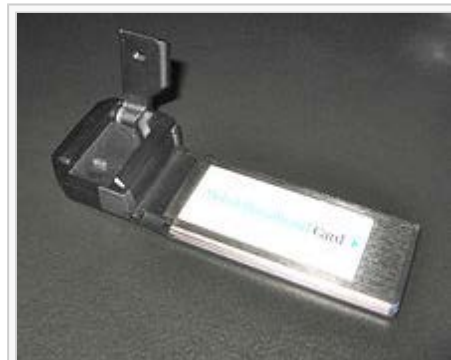
A mobile broadband modem in the ExpressCard form factor for laptop computers
