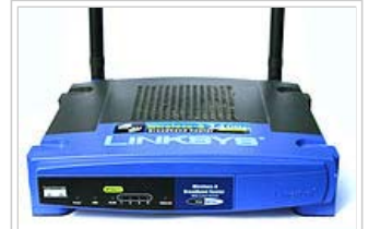
The Linksys WRT54G contains a router with an 802.11b/g radio (common in the early 2000s) and two antennas
