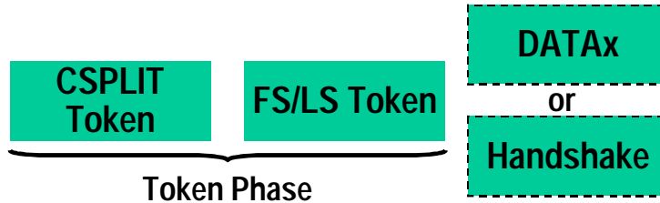
Figure 8-7. Packets in a Complete-split Transaction
