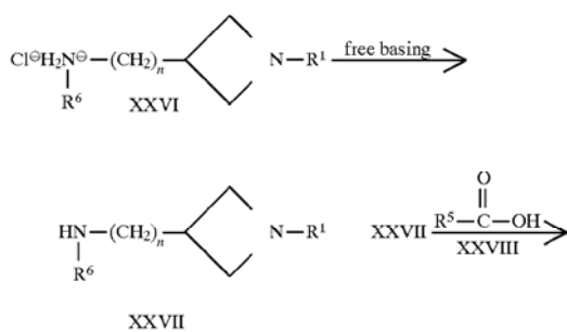
Scheme XI Preparation of Compound II (Robotic Amide Coupling)
