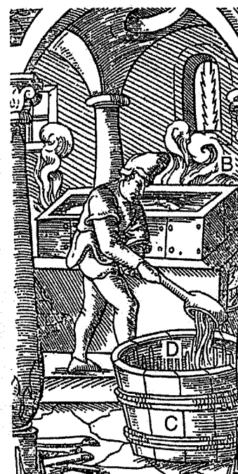
Figure 8.1 Borax refining in the sixteenth century, (D) copper rods, and (E) grinding. (From Borax Inc.)
