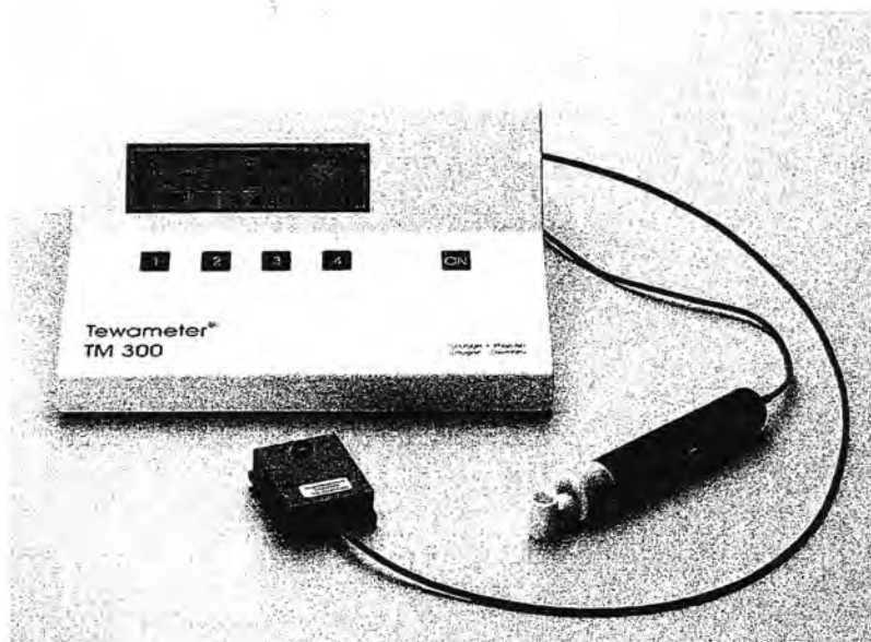
FIGURE 7.1 Tewameter for measuring transepidermal water loss in skin. (Courtesy of Courage + Khazaka electronic GmbH, Köln, Germany.)
