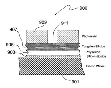
Figure 9 depicts substrate 901 having a stack of layers including oxide layer 903, polysilicon layer 905, tungsten silicide layer 907, and photoresist masking layer 909 with opening 911, from the treatment method shown in Fig. 10, below. *Id.* at 17:58–18:57.
