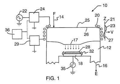
Figure 1 depicts a substrate (product 28, such as a wafer to be etched) on a substrate holder (product support chuck or pedestal 18) in a chamber (chamber 12 of plasma etch apparatus 10). *Id.* at 3:24–25, 3:32–33, 3:40–41.
