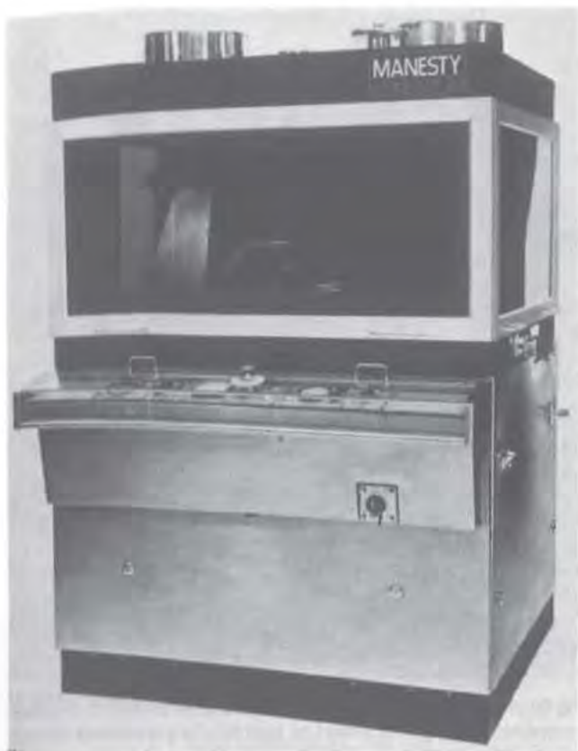
Fig 90-21. Rotapress Mark II A; designed for improvements in sound reduction, operator safety, cleanliness, and operational convenience; note control panel on front of machine (courtesy, Thomas/Manesty).
