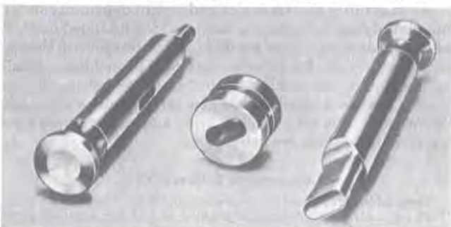
Fig 90-2. Basic mechanical unit for tablet compression: lower punch, die, and upper punch (courtesy, Vector/Colton).
