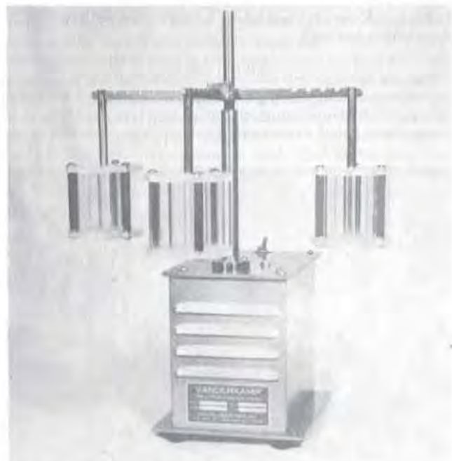
Fig 90-5. Vanderkamp Tablet Disintegration Tester (courtesy, Van-Kel).
