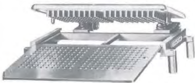
Fig 90-28. Tablet triturate mold (courtesy, Vector/Colton).
