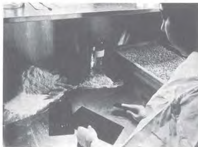
Fig 90-27. Hand molding tablet triturates (courtesy, MSD).
