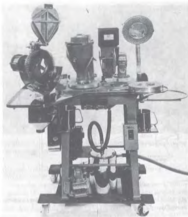
Fig 90-36. Type 8 capsule-filling machine (courtesy, Lilly).
