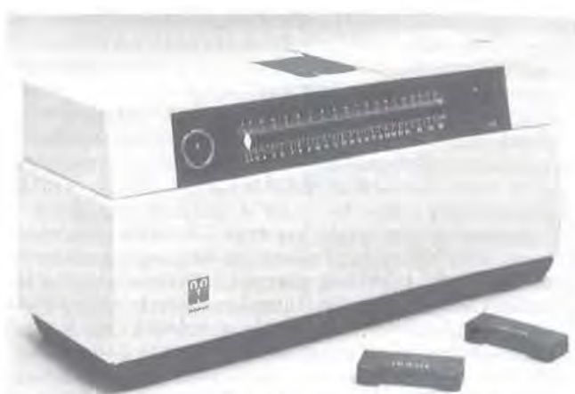
Fig 90-3. The Schleuniger or Heberlein tablet hardness tester shown with calibration blocks (courtesy, Vector).
