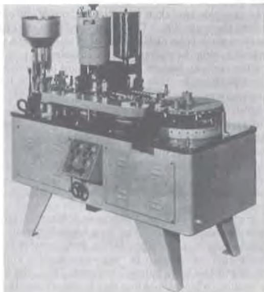
Fig 90-37. MG-2, automatic capsule-filling machine (courtesy, Supermatic).
