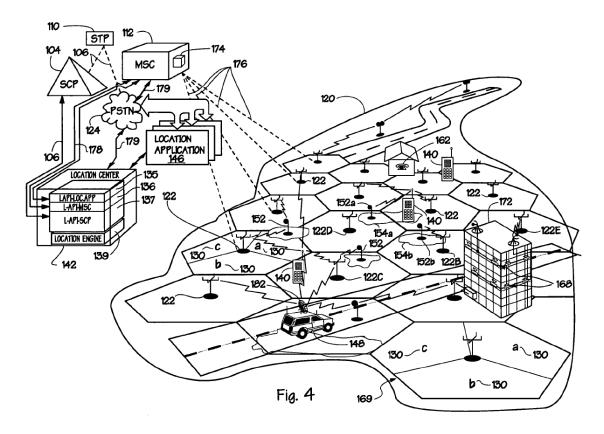
Figure 4 is an overall view of a wireless radio location network architecture. *Id.* at 21:66–67. The network includes a plurality of mobile stations ("MS") 140, a mobile switching center ("MSC") 112, and a plurality of wireless cell sites forming radio coverage area 120, each site including a fixed-location base station 122 for voice and data communication with MSs 140. *Id.* at 24:41–57. The network also includes location base stations ("LBS") 152
