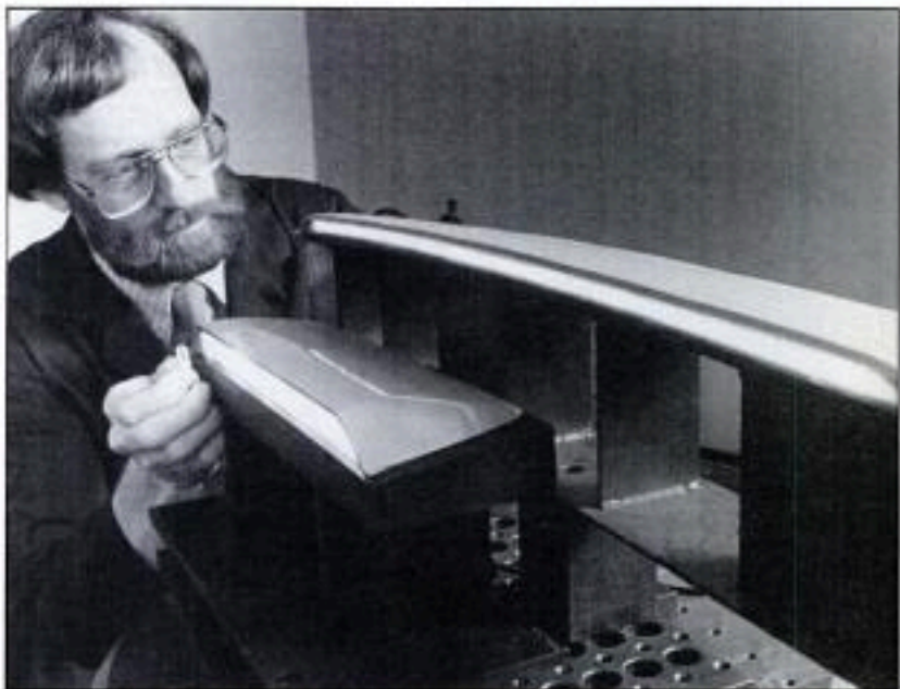
The LED's tiny size helps streamline a center-mounted automobile brake light.
