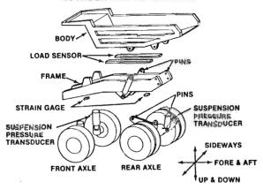
The running gear: it is possible to attach strain gauges to the running gear or in the running gear mounting pins, however, these strain gauges are very susceptible to damage and do require ongoing calibration. Further as the rear axle, in particular, oscillates its relative position to the truck frame changes throwing meaningful load weighing way out of wack. (Fig 5)
