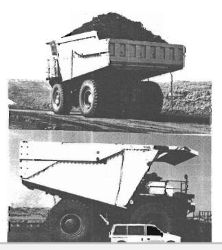
Providing the point is made for the need to weigh trucks, how can an on board truck weighing system be installed? Separating a truck into discrete components: 1) running gear, front axle and rear axle, 2) the truck frame, and 3) the truck body. These are the areas at which a truck can be weighed.
