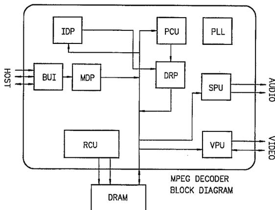
processor, an image data processor, an inverse transform and reconstruction processor, and a prediction calculation unit. A video post-processing unit generates video data, and a serial
