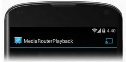
Figure 2. A Cast button shown on the right side of the action bar.
