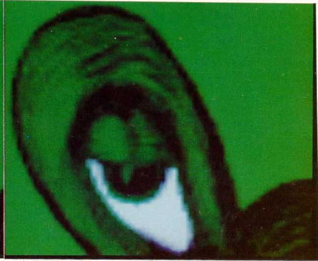
Figure (4) Upsampling the frog: magnification by bilinear interpolation.
