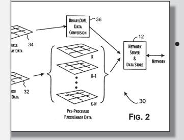
"In accordance with the preferred embodiments of the present invention, as generally illustrated in FIG. 2, a network image server system 30 stores a combination of source image data 32 and source overlay data 34. The source image data 32 is typically high-resolution bit-map satellite imagery of geographic regions, which can be obtained from commercial suppliers." (Ex. 1001, 5: 54-67) (Paper 2 at 7, Paper 27 at 2, Ex. 1008, ¶ 81)
