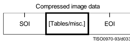
Figure B.15 – Abbreviated format for table-specification data syntax
