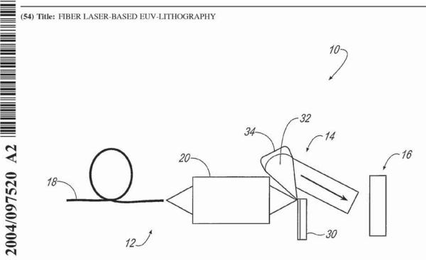
(57) Abstract: A method and apparatus is disclosed for performing lithography operation. A fiber laser (18) is provided that generates laser light that is used by adaptive optics (20) to focus the laser light onto a plasma target (30) to generate plasma as a source
