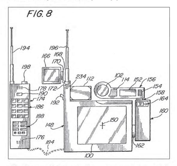
100. Moreover, McNelley also discloses a cellular telephone: "[i]n the near future, video-phone networks will use one or a combination of phone lines, television cables and wireless networks (i.e., cellular phone systems). The telecamcorder is applicable to any type of network." *Id.* at 14:16-18. McNelley discloses the telecamcorder "where the camera 102 is pointed in the same direction
