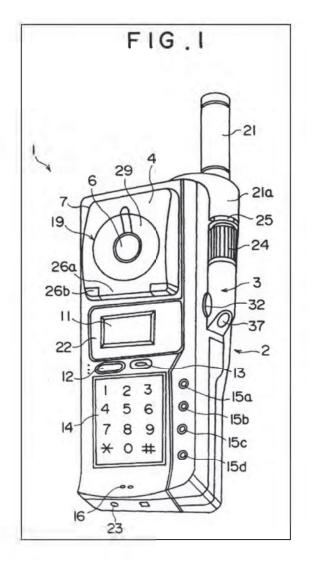
111. Umezawa discloses that the video telephone contains "the display panel 11 which is comprised of a liquid crystal" and depicted in Fig. 1 above. *Id.* at 5:59-60. Umezawa discloses that:
