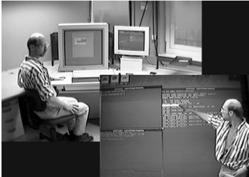
Fig. 7: View of the HDMM Lab and Demo Center with high-resolution display (2k x 2k) and rear projection for conferencing applications
