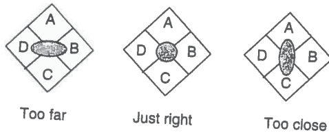
Figure 12.51 The separation between the laser and the compact disk is critical for the correct operation of the CD player. A clever astigmatic autofocus mechanism is used to maintain this distance.
