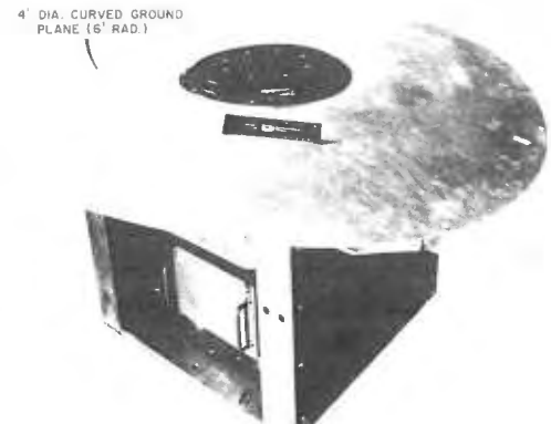
Fig. 5 Eight-Element Circular Array Antenna/Steering Electronics
