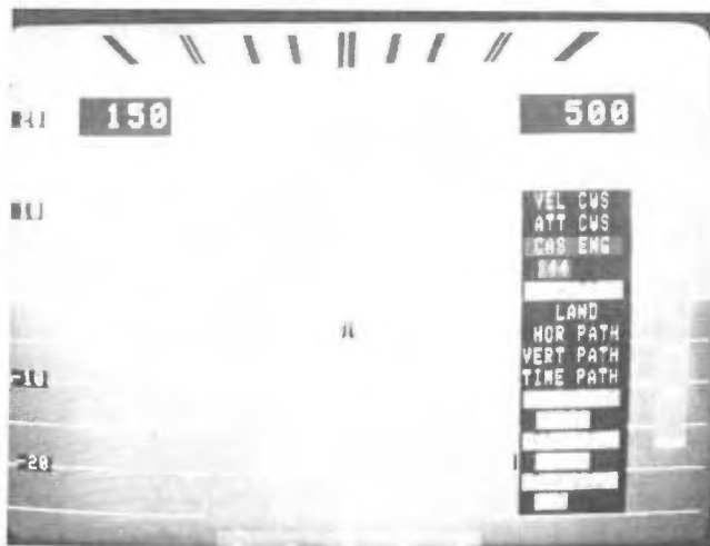
Fig. 5 PFD (EADI) with menu implementation of AGCU functions.
