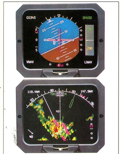
Electronic altitude director (top) and horizontal situation indicator
