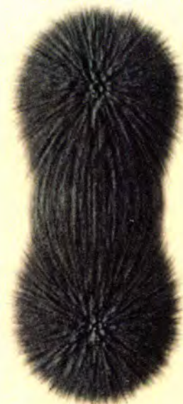
Figure 14: A three-dimensional 512^3 electrostatic field is imaged by volumetrically ray tracing a three-dimensional scalar field produced using LIC over white noise.
