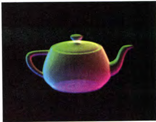
Figure 8: Utah teapot. Frequency domain volume rendering. The pot is lit by a red light (right), a green light (upper left), and a blue light (lower left).
