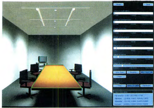
Figure 5: Sample interface which allows the user to set the weights of the objective and/or specify constraints.
