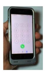
a charger plug integrally formed with the charger and located on the charger such as to allow the charger plug to be inserted into a charging port of the mobile device, The Squirl case has an integrally formed male portion of an electrical fitting that is configured to be inserted into a female socket in an iPhone when the iPhone is placed into the case.
