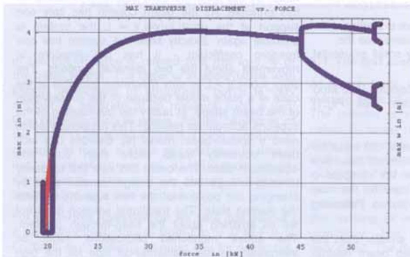
Fig 8 Time-process of the maximal deformation at x = L/2 red line: represents the traditional solution blue line: represents the w-F-w-scenario start displacement: 1 m start time-step \Delta f of the force process: 10^{-13} kN
