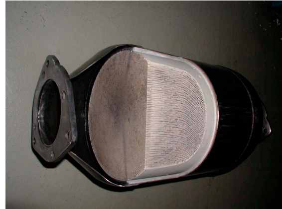
Figure 3. 2-way SCR/DPF hardware
