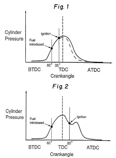
Figures 1 and 2 depict graphs showing the cylinder pressure-crankangle characteristics for a typical direct injected two-stroke internal combustion engine and for such an engine operated according to the method of the '365 patent, respectively. *Id.* at col. 2, ll. 46–52.
