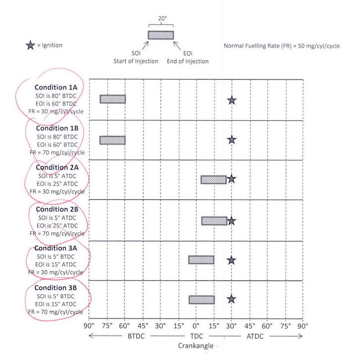
1. A method of operating an internal combustion engine comprising retarding the ignition of a gas/fuel mixture within at least one cylinder of the engine to after top dead centre (ATDC) in respect of the combustion cycle of said at least one cylinder of the engine. For THE OCHAINAL SUBMISSION OF CLAIM 1
