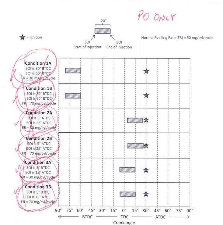
1. A method of operating an internal combustion engine comprising retarding the ignition of a gas/fuel mixture within at least one cylinder of the engine to after top dead centre (ATDC) in respect of the combustion cycle of said at least one cylinder of the engine.
